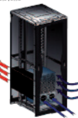
Figure 1. NET-ACCESS ® Cabinet Thermal Duct Air Circulation
