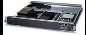
WebVPN Module for 6500/7600 ~300Mbps, 8000 Users (4 blades Per Chassis – 32k users w/ 1.2 Gig of Throughput)
