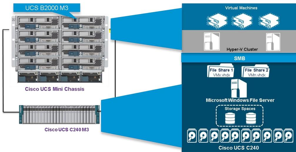
Figure 3 shows the logical design of the proposed solution. The Cisco UCS C240 M3 is configured as the Microsoft Windows SMB file server. The Cisco UCS 240 M3 can host up to 24 SFF SAS disks, which can be both SSD and SAS disks. Storage Spaces uses tiering to achieve optimal performance. In the design, three virtual disks are configured using an LSI MegaRAID card on the Cisco UCS C240 M3. A RAID 1 virtual disk is used for hosting the Windows Server 2012 R2 OS for the Cisco UCS C240 M3.
