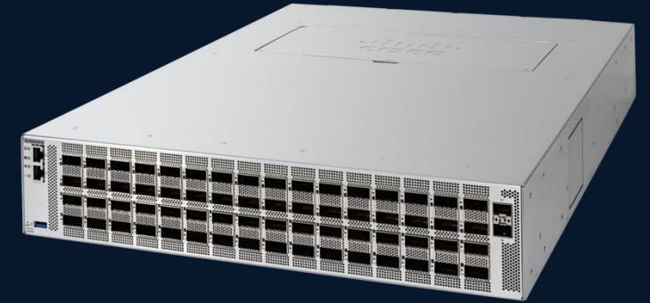
N9364E-SG2X-Q 64p 800G QSFP-DD 2RU
