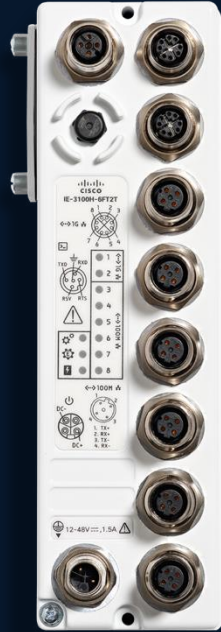
IE3100H FE/GE 6x FE (D-Code M12) 2x GE (X-Code M12)
