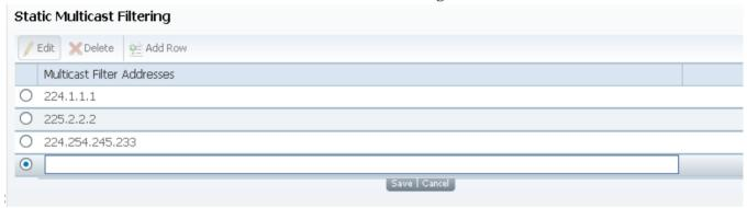
**2** Type the IP Address that sets the destination for multicast MPE data, in the range from 224.0.0.0 to 239.0.0.0.
