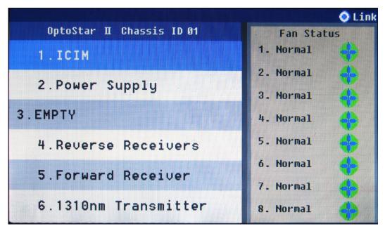
As shown in the illustration, all the local modules are located on the left side of the screen, you can press ▶ button to move to the next page, and view modules in other slots. The statuses of 8 fans are located on the right side of the screen.
