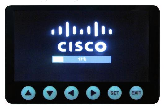
3. When the device initialization is complete, remove the ICIM display and begin operation.
