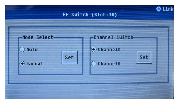
Factory default sets switching mode to Auto. By default, the cursor is set on the Auto option and the module is set to work in auto switching mode. Press ▲ ▼ button to select auto or manual switching mode.
