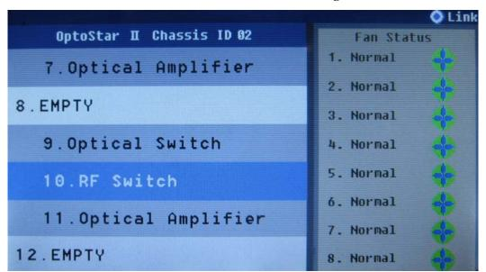
Press ▼ button to move the cursor down to RF Switch (OptoStar II RF switch module), and press the SET button to enter the sub-menu of the RF switch.
