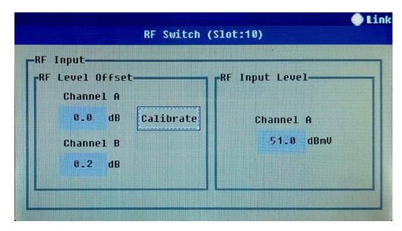
The RF input information shows/sets input level calibration and shows the RF input level value of channel A.
