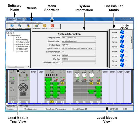
The OptoStar II console main interface shows the software name, menus, menu shortcuts, local module tree view, system information, chassis fan status, and local module view.
