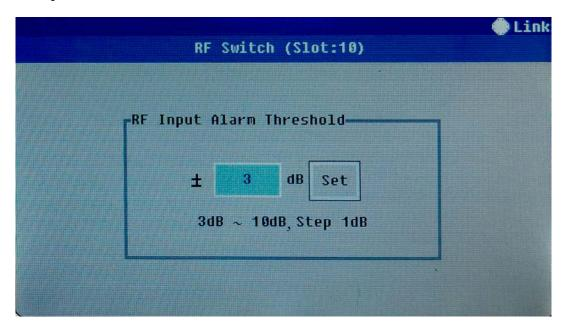
The default value of RF input alarm is 3 dB. In auto switching mode, if the calibrated signal value is out of this range, the module will alarm and perform auto switching according to different conditions (refer to Page 3-7).
