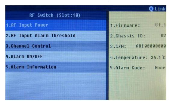
The left side of the screen shows the sub-menus of the OptoStar II RF switch module. By default the cursor is on sub-menu 1. Press ▼ button to move the cursor down. Press SET button to enter the item on the sub-menu.
