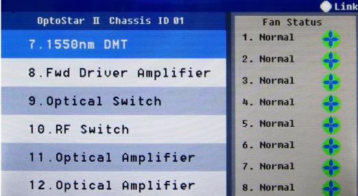
As shown in the illustration, all the local modules are located on the left side of the screen, you can press ▶ button to move to the next page, and view modules in other slots. The statuses of 8 fans are located on the right side of the screen. When the left Link circle at the top right corner lights in blue, it indicates connection of RJ-45 cable; if the light is off, it indicates no connection.
