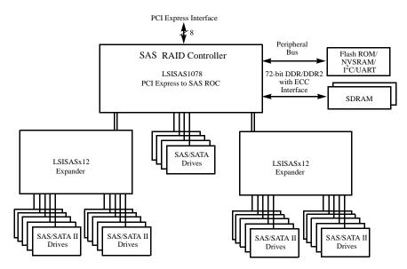
Figure 2: Example of an LSI SAS RAID Controller Configured with an LSISASx12 Expander
