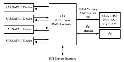
Figure 1: Example of an LSI SAS Direct-Connect Application
