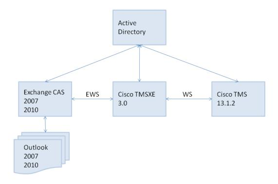
Cisco TMSXE communicates with Exchange 2007 or Exchange 2010 using Exchange Web Services (EWS).
