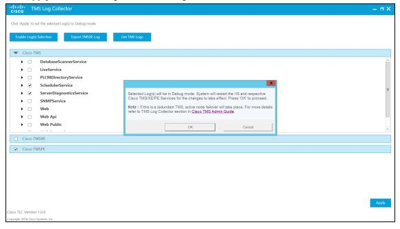
Click OK. The logs are set to debug mode and the system restarts the IIS and respective Cisco TMS/TMSXE/TMSPE services. Reset To Initial button is enabled.
