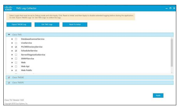
5. If you try to close the tool when it is in Debug mode, it will not allow you to close unless you reset the logs to their original mode.
