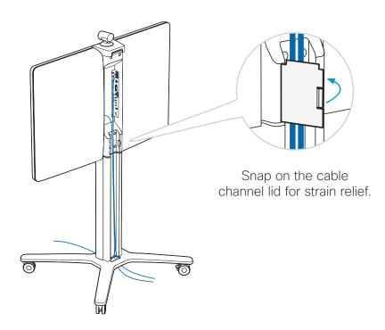
Lead the cables out at the front or back as appropriate.
