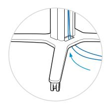
Thread the cables up through the hole in the base.
