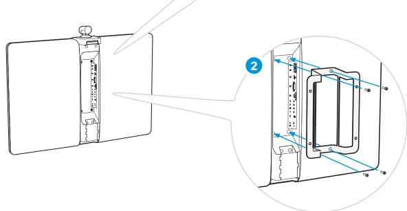
Fasten the bracket with the four screws that you just removed.
