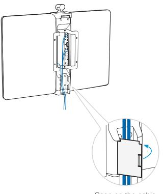
Snap on the cable channel lid for strain relief.
