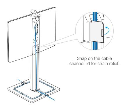
Lead the cables in the cable slots. Lead them out at the front or back as appropriate.
