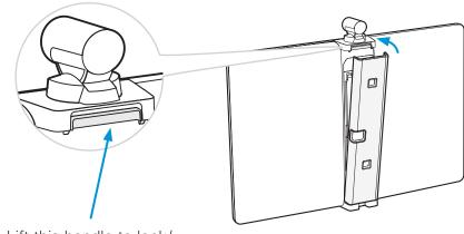
Lift this handle to lock/ unlock the back cover. Use both hands if required.
