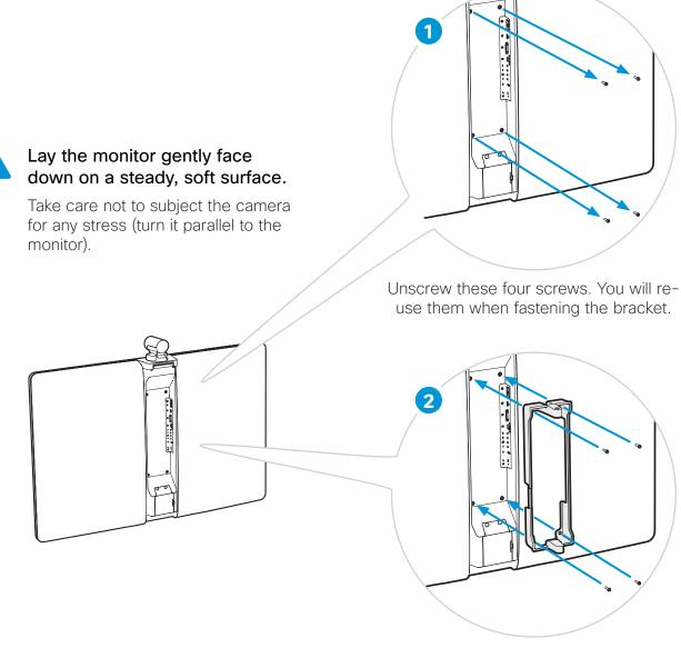
Fasten the bracket with the four screws that you just removed.
