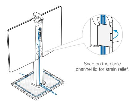
Lead the cables in the cable slots. Lead them out at the front or back as appropriate.
