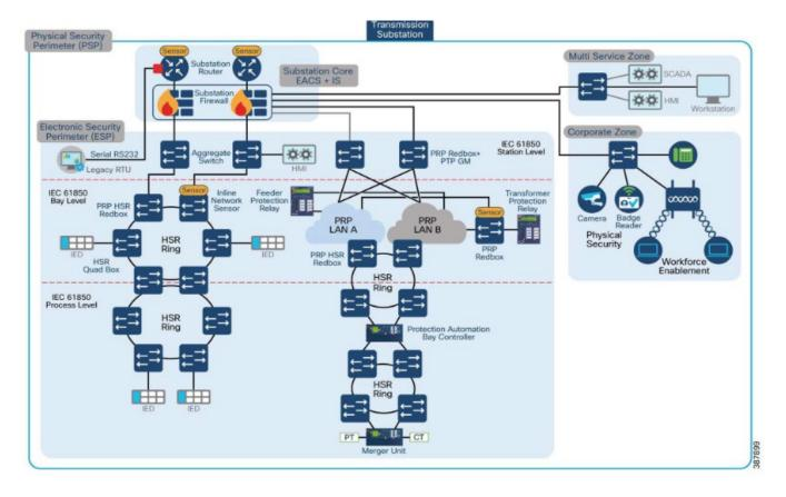
The Cisco new digital substation architecture comprises an operations and control center, demilitarized zone, WAN tier, transmission Substation Physical Security Perimeter (PSP) and WAN connectivity for other secondary substations, and local multiservice and corporate networks. The PSP is divided into substation core, Electronic Security Perimeter (ESP), and Multiservice and Corporate (CORP) zones. Based on the IEC 61850 standard, ESP is further subdivided into station, bay, and process Levels.
