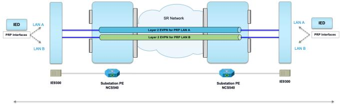
Teleprotection Circuit 5ms/200us Asymmetric delay (Maximum 20 Hops , 500Km Fiber)
