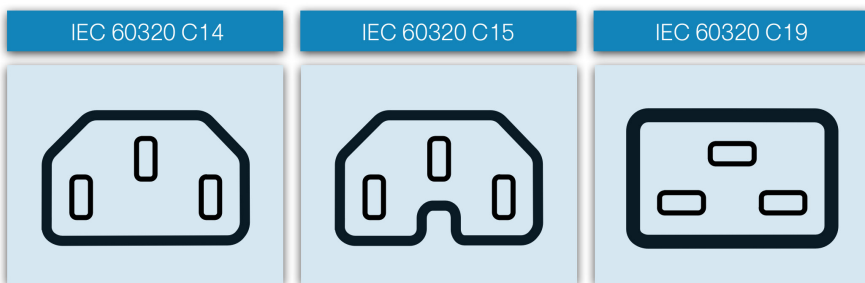
Figure 3 - Plug types used by Cisco devices
