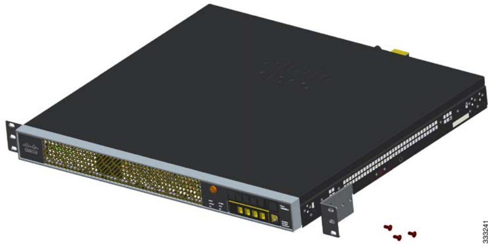
Figure 3-3 Attaching the Rack-Mount Brackets
