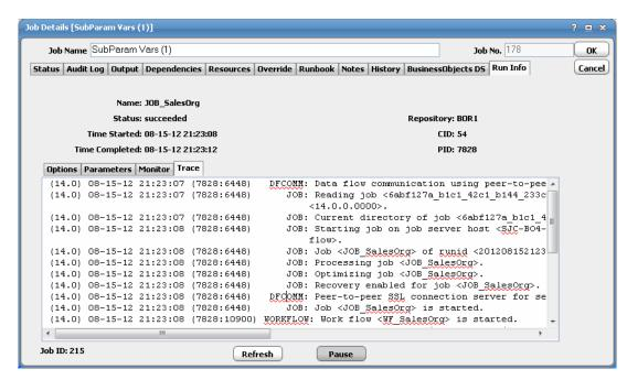
Use the trace logs to determine where an execution failed, whether the execution steps occur in the order you expect, and which parts of the execution are the most time consuming.
