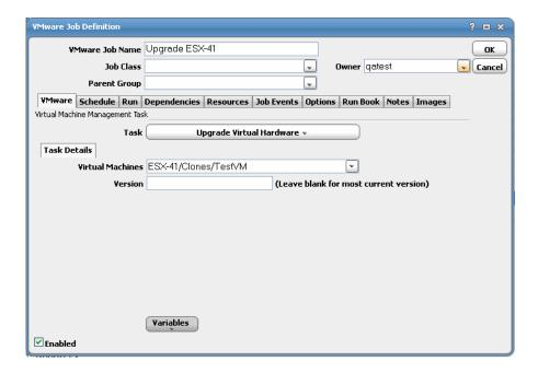
• Virtual Machine - Name of the virtual machine to be upgraded
