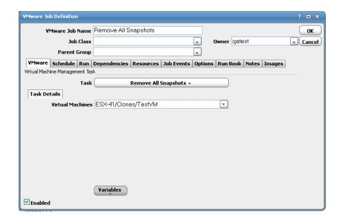
• Virtual Machine – Name of the virtual machine on which the snapshots were taken.
