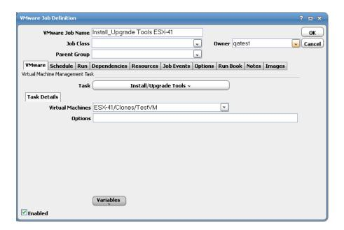
• Virtual Machine – Name of the virtual machine on which to install or upgrade the VMware tools.
