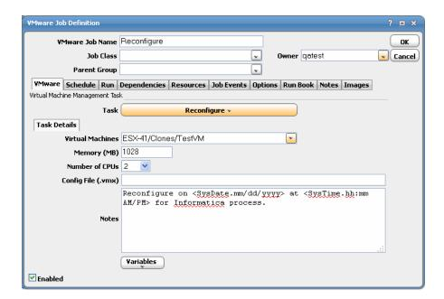
• Virtual Machines – Name of the virtual machine to be reconfigured.
