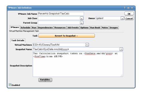
• Virtual Machine – Name of the virtual machine on which the snapshot was taken.
