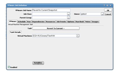
• Virtual Machine – Name of the virtual machine on which the snapshot will be reverted.
