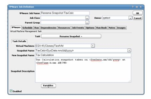
• Virtual Machine – Name of the virtual machine on which the snapshot was taken.
