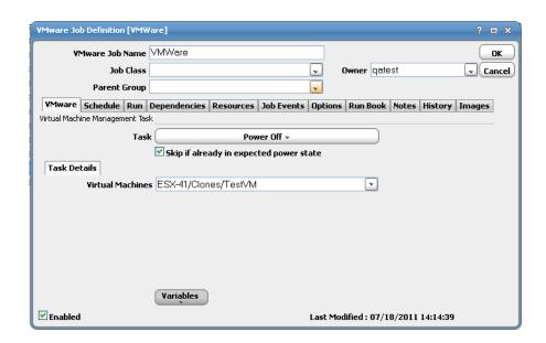
• **Skip if already in expected power state** – Select this check box if you want the job to complete normally if the virtual machine is already powered off.
