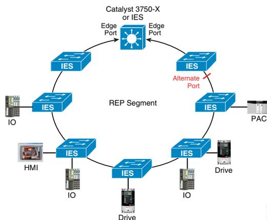
REP intelligence prevents the creation of a traffic loop condition when a ring of the Stratix 5700/8000 series switches is utilized. If a cable breaks or switch service disrupts, REP allows CIP traffic to continue to reach the edge of the ring topology for IACS, monitoring, and management continuity.
