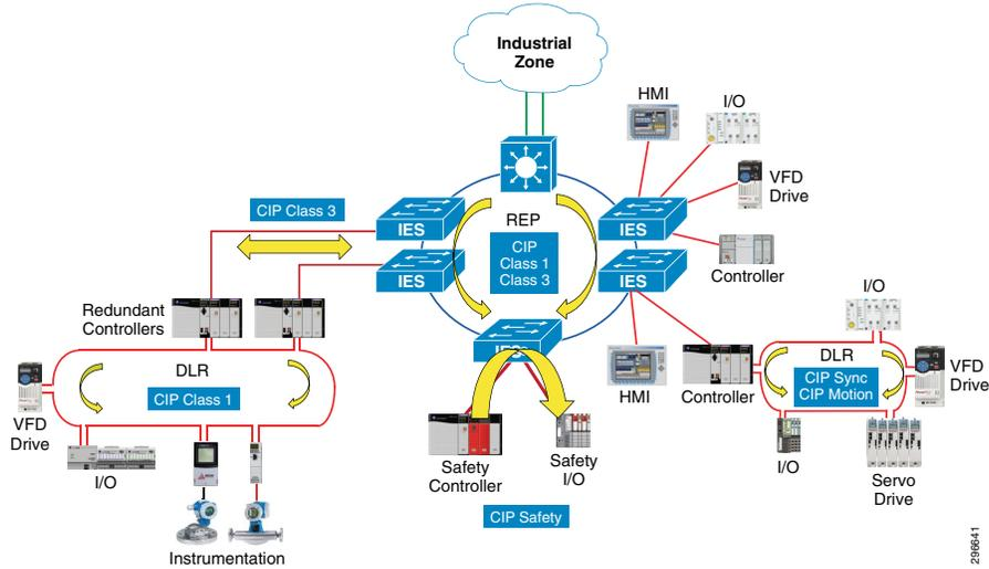
The REP architecture aligns with previous CPwE systems from an overall architecture framework (Figure 2) perspective and with general design and implementation recommendations in order to continue to align with industry standards. The REP architecture utilizes EtherNet/IP™ network communications, which are driven by the ODVA Common Industrial Protocol (CIP).
