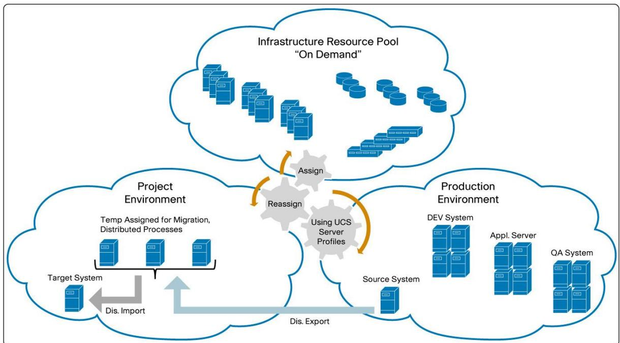
The Cisco Unified Computing System allows customers to assign and reassign infrastructure resources on-demand, when and where they are needed. This enables administrators to support their projects and day-by-day operations without laborious and time-consuming configuration tasks while providing additional capacity to their SAP environment.
