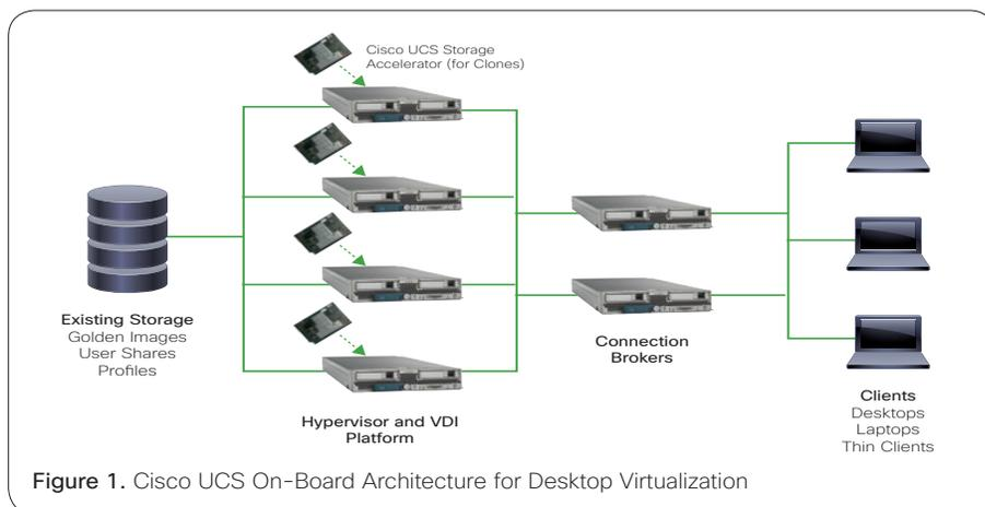
Figure 1. Cisco UCS On-Board Architecture for Desktop Virtualization
