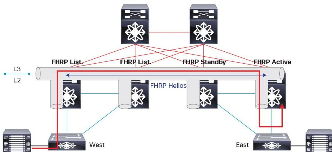
[Figure 3](#) shows the deployment of independent default gateways in each data center site to optimize and localize routing of outbound traffic flows.
