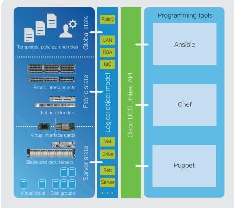
Figure 1 The unified API provides programming tools with access to all Cisco UCS resources
