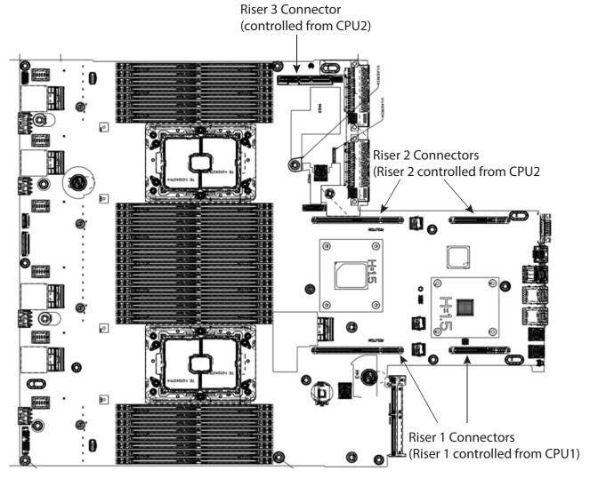
Figure 9 shows the locations of the PCIe riser connectors on Cisco UCS C240 M7 SFF motherboard.
