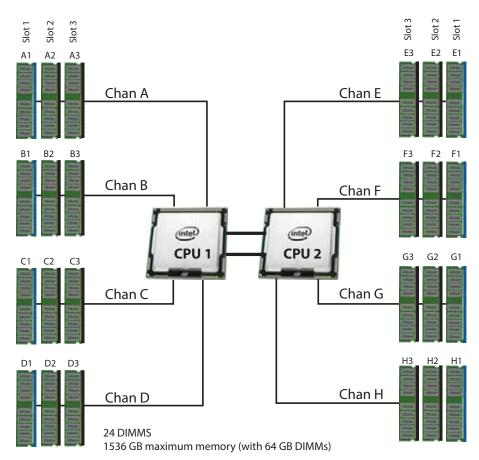
4 memory channels per CPU, up to 3 DIMMs per channel
