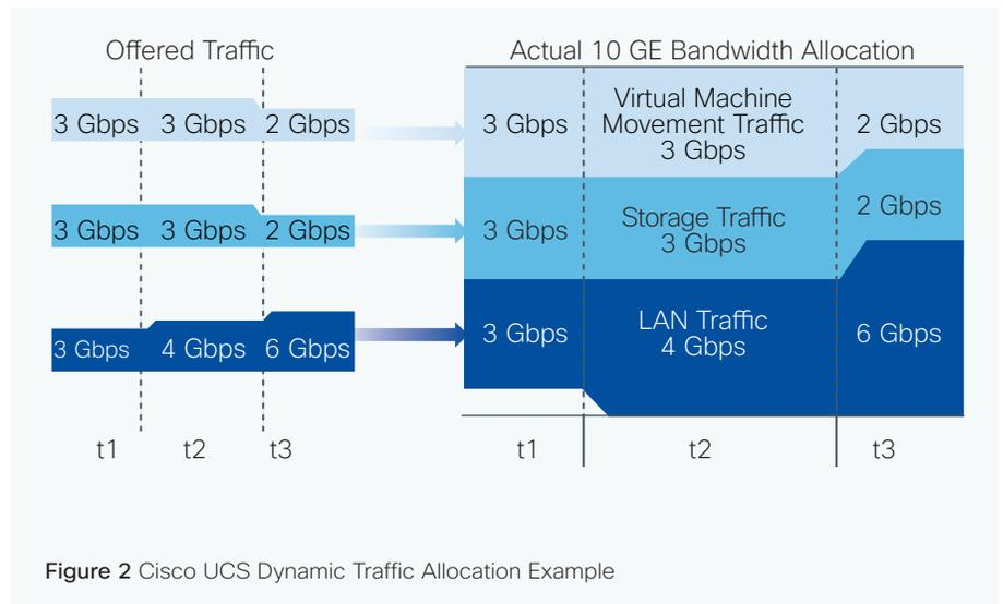
Figure 2 Cisco UCS Dynamic Traffic Allocation Example
