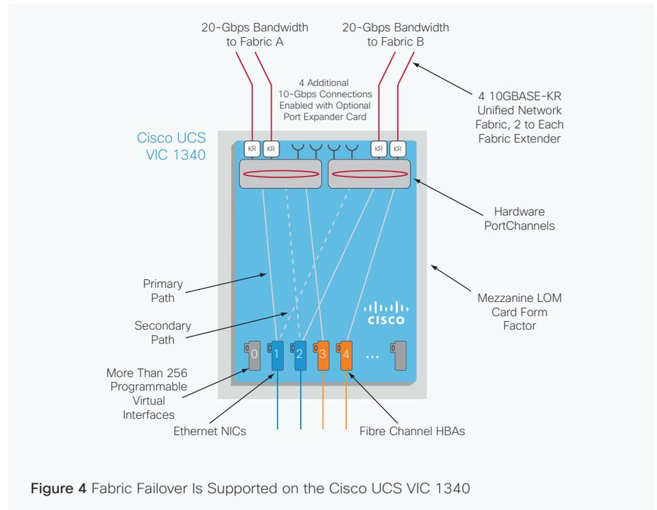
Figure 4 Fabric Failover Is Supported on the Cisco UCS VIC 1340
