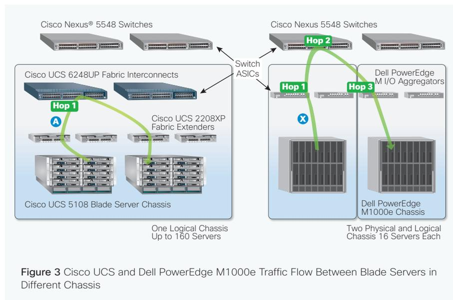
Figure 3 Cisco UCS and Dell PowerEdge M1000e Traffic Flow Between Blade Servers in Different Chassis
