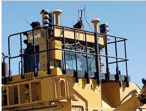
Figure 52 Example of Dozer with a Single Radio and OMNI-5-KIT Antenna installed on the top
