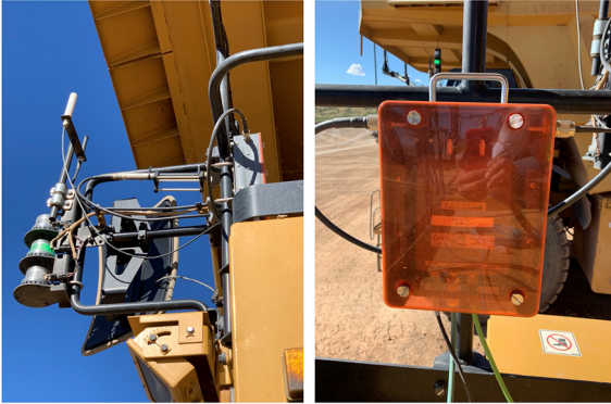
Figure 49 Example FM4500 and OMNI-KIT-5 Antenna installation on the side of a Haul Truck
