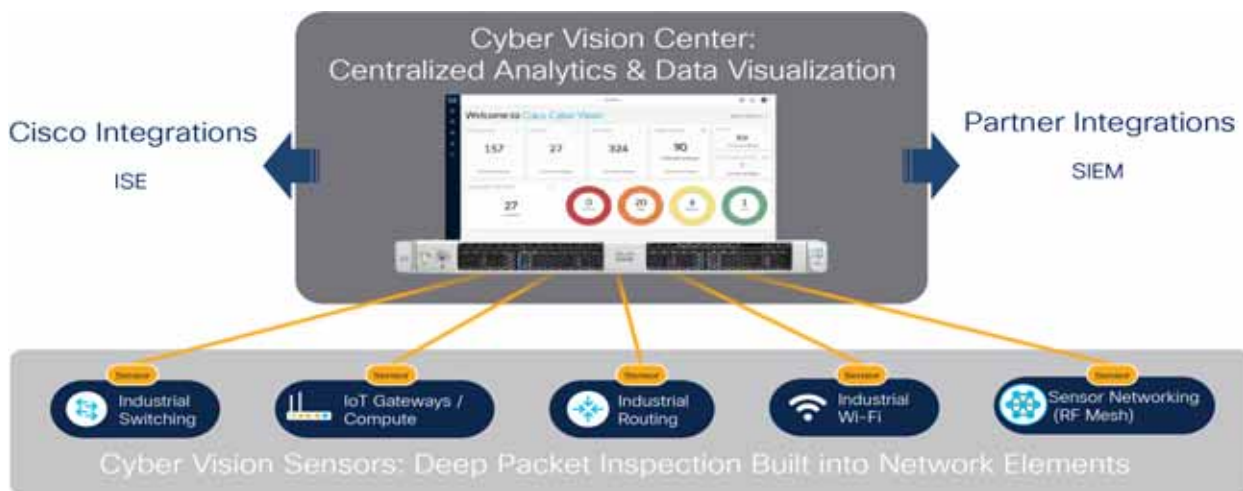
Figure 65 Cisco Cyber Vision Two Tier Architecture
