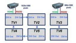
These dedicated DMPs provide the video signal for the group of TVs that the DMP is connected to through the daisy-chain. Depending on the screen manufacturer, the RS-232 connections can also be daisy-chained if this feature is available.
