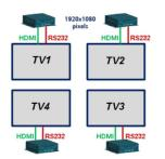
This cabling method also is required for zone-based synchronization, which is recommended to achieve enhanced functionality for dedicated video walls running videos with a duration greater than 15 minutes.
