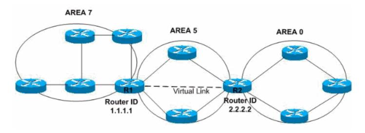
In this example, the virtual link is created between the routers with router ID 10.1.1.1 and router ID 10.2.2.2. In order to create the virtual link, configure the **area 5 virtual-link 2.2.2.2** subcommand on router 10.1.1.1 and the **area 5 virtual-link 1.1.1.1** subcommand on router 10.2.2.2. Refer to <u>Configuring OSPF Authentication on a</u> <u>Virtual Link</u> for more information.
