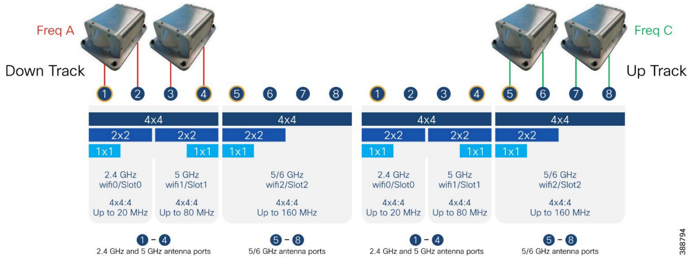
Figure 19 Onboard train dual frequency dual radio antenna connections
