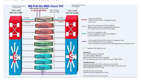
M4/M5 Micropod with Intel NIC (X710) - NIC Redundancy
