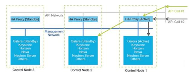
In the figure, Control Node 1 is attached to the API network segment through the br\_api bridge. The br\_api bridge connects to the Linux network namespace where the HAProxy container has an interface that is mapped through the api < > api\_out interface mapping. The HAProxy container has a default gateway configured that points to the upstream API Layer 3 First Hop Redundancy Protocol (FHRP) VIP. This gateway is used for the HAProxy container incoming and outgoing API traffic.
