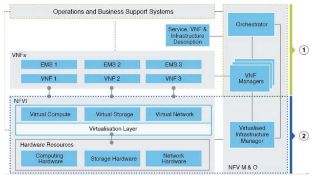
At a high level, the NFVI architecture includes a VNF Manager and NFV Infrastructure.
