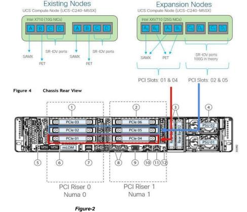
Both configurations displayed in *Figure-1* and *Figure-2* on UCS C240 M5SX server are supported Configurations.
