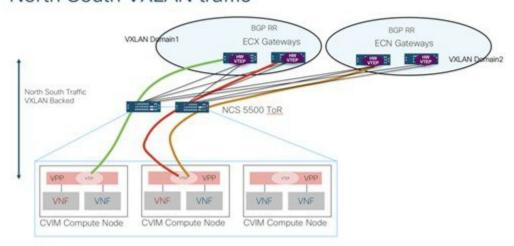
One set of VXLAN overlays manage the Cloud exchange traffic, while the other set of VXLAN overlays manage the Cloud management traffic. The multi-VXLAN (multi refers to 2) is used to conserve the number of bridge domains (BD) consumed on the Cisco NCS 5500 ToR.
