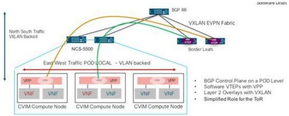
From a control plane point of view, three instances of GoBGP (in Active-Active mode) run on the controller nodes to establish L3 peering with the external BGP RR for importing or exporting VxLAN routes into or from Cisco VIM respectively. The imported information is then pushed into etcd, to maintain a single source of the information within Cisco VIM.
