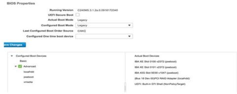
If the boot order for the Intel NICs is not listed as above, enable the PXE boot setting for each UCS-C M4 series server by using either Intel's BootUtil tool on a pre-installed Linux system or boot a special ISO image. This is time consuming especially on a large pod with many nodes. Hence, an automated tool is developed to help with this painstaking process.
