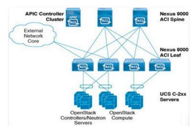
The Opflex ML2 plugin integrated with Cisco VIM in Unified mode manages the tenant VLANs dynamically, as and when the VMs operate in the cloud. By utilizing OpFlex, the policy model native to ACI can be extended to virtual switches running on OpenStack Nova compute hosts. OpFlex extension to the compute host allows ACI to use Open vSwitch (OVS) to support common OpenStack features such as Source NAT (SNAT) and floating IP in a distributed manner
