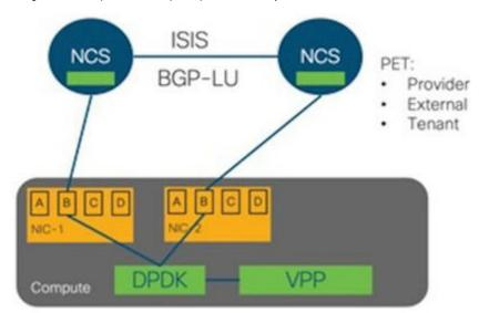
The VPP backed data plane ports are configured differently. Each NIC has a port connected to one NCS. This link is a routed link with an IP address both on the NIC port in the Cisco VIM node and an IP address on the NCS port. These addresses come from a /30 subnet. ISIS runs between the NCS and BGP-LU. On the Cisco VIM nodes, ECMP load balancing occurs over the two links to the NCS. On VPP, there is a loopback interface configured that is used as the SR node SID.
