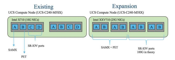
For computes with 25G NICs, the lower two NIC slots are used for control and data plane. Hence, care must be taken in placing the NICs across the NUMA node. In an UCS 240 M5 node, use slot 1 for the first 25G NIC, and slot 4, 5, and 6 for next 3 25G NIC cards to yield a balanced virtual network across NUMA nodes. However, SRIOV is dedicated to a single NUMA.
